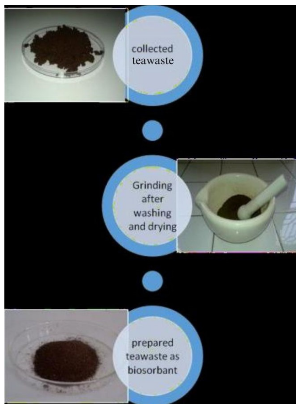
Figure 1. Preparation of biosorbent tea ( Camellia sinensis ) waste.
